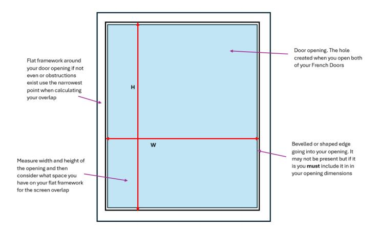
Measure the width and height of the opening including any bevelled edge on the door frame going into the opening and add 40mm to each measurement. This will give you a 20mm overlap on the door frame either side (i.e. half the width of the screen frame).
